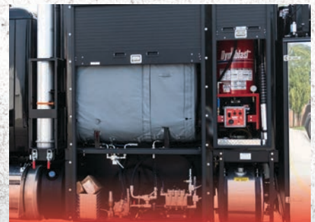
Insulated Enclosure Houses Blower & Water Pump
