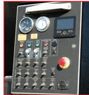
Main Controls with E-Stop
